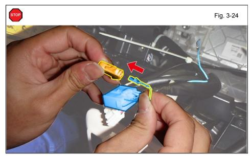
al. Insert the V5 Sky Blue Wire Terminal into the indicated location on the 10P Vehicle Connector. (Fig. 3-24)
