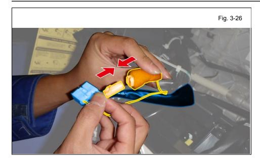
an. Connect the V5 White 1P Connector to the V5 White 1P Connector. (Fig. 3-26)
