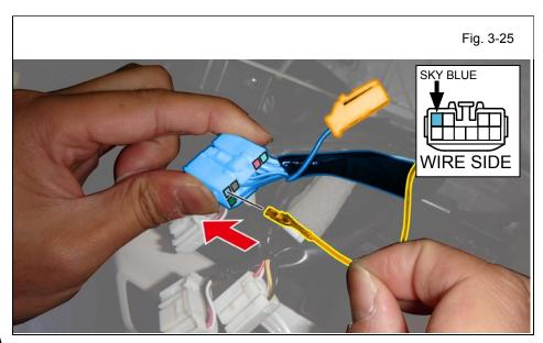
am. Connect the V5 White 1P Connector to the V5 White 1P Connector. (Fig. 3-25)
