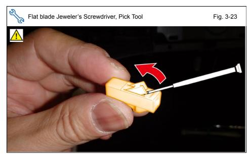
ai. Lift the Terminal Retainer Clip. (Fig. 3-23)
