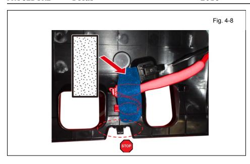
k. Apply 1 Foam Tape to the GBS Microphone as shown. (Fig. 4-8)
