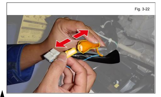
ah. Disconnect the V5 White 1P Connector from the V5 White 1P Connector. (Fig. 3-22)
