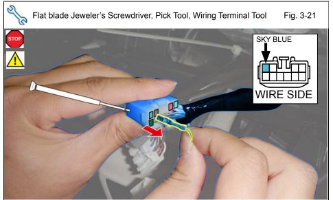
ag. Pull out the Vehicle's Sky Blue Wire Terminal from the indicated location on the 10P Vehicle Connector. (Fig. 3-21)
